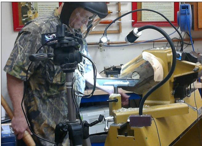
Kevin has the blank mounted and has begun turning. Here he’s stopped the lathe to inspect the cut before proceeding.
