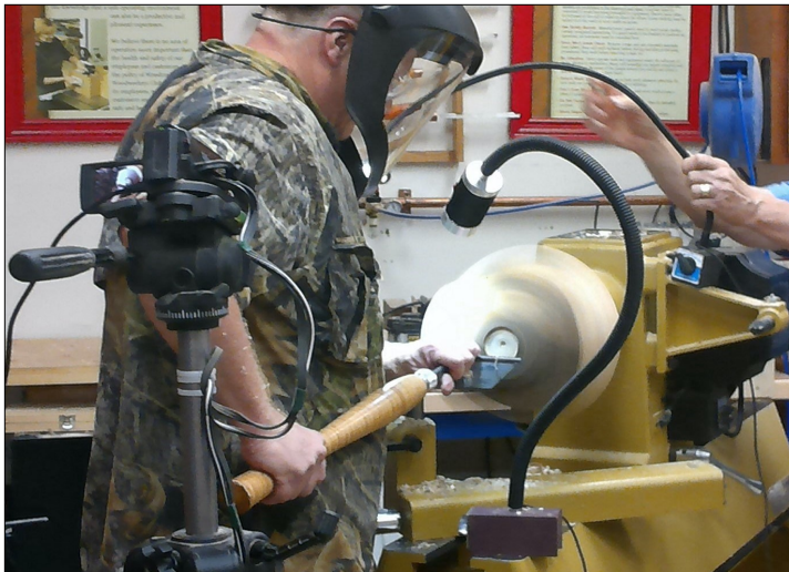
Hollowing has begun. Here you can see Hans holding the second light. Two lights are used to assist on the interior work.
