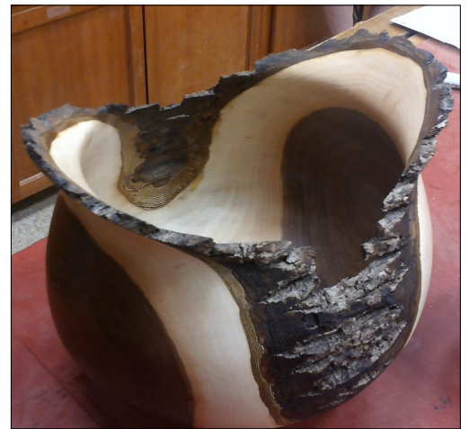
Kevin has the blank mounted and has begun turning. Here he’s stopped the lathe to inspect the cut before proceeding.
