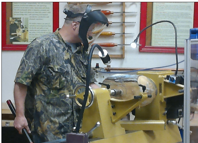
Blank is mounted and OD turning begun
