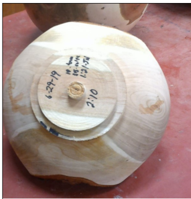
Date and process step duration time is recorded for each piece. Kevin uses this information to help control the fabrication process for each bowl.
