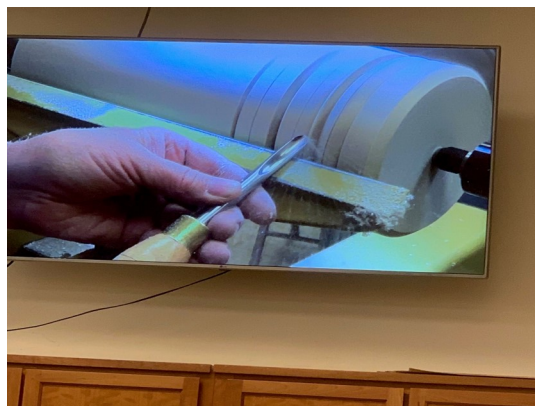
Or use a gouge for the bead
