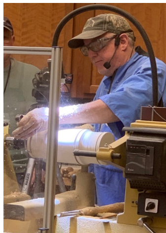
Starting the turning by sizing the wing diameters
