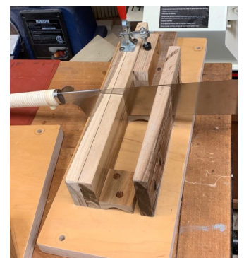
One of the custom made jigs for cutting blanks by "touch"
