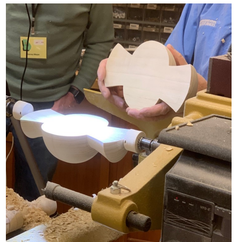
"Halving" the blank by turning the trunnion (handle) diameters to size
