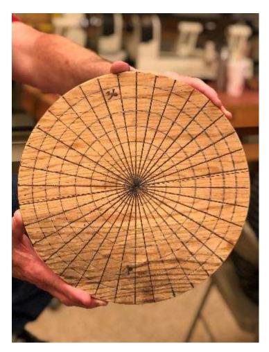
Index plates are used to lay out the flute spacing and texture blocks after the bowl is roughed out. The bowl can be laid on the plate and quickly divided. Shown here is a 36 segment plate. The radial lines are bisected with rings that can be used to center the object on the plate and index spacing as desired.
