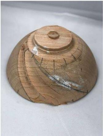
One the blank has been marked with index lines, Al selects an off-set value to set the pitch for the "helical curve". The curve is laid onto the bowl surface using a gauze plaster bandage that marks the curve. The bandage dries quickly and is transferred between index points to enable creation of uniform layout lines. Much faster than hand plotting each curve!
