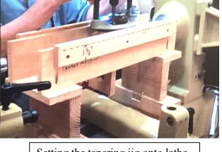
Setting the tapering jig onto lathe
