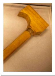
Handle blank assembled onto top section of shaft
