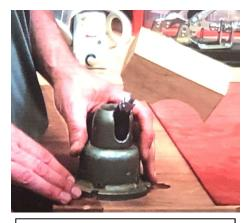
Handle blank mounted in swivel vise enables easy access for shaping
